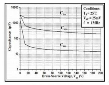
Figure 15. Capacitances vs. Drain-Source Voltage (0 - 200V)
