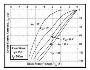
Figure 13. 3rd Quadrant Characteristic at 25C
